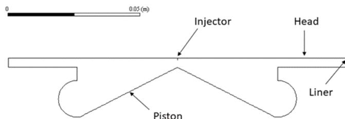
**Fig -1:** Combustion Chamber of single cylinder research engine at TDC
