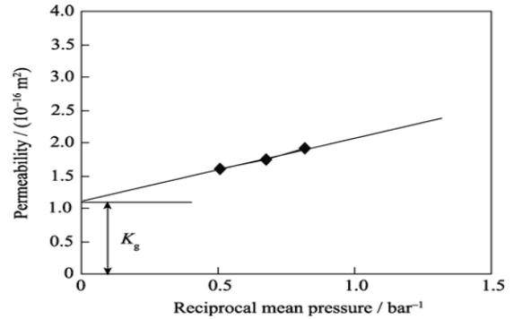
Fig. 2. Relationship between permeability and reciprocal mean pressure.
