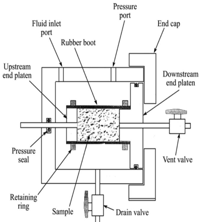
Fig. 1. Cell and specimen holder
