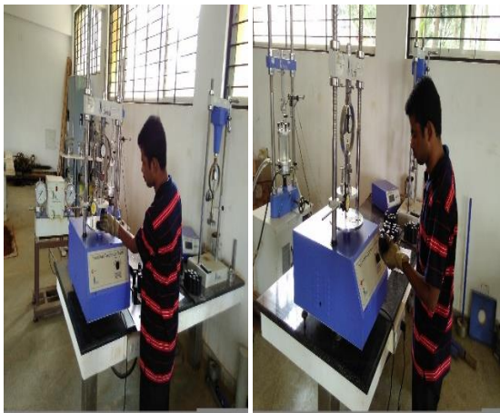
Figure 5.6, 5.7 Conducting Unconfined Compression Test
