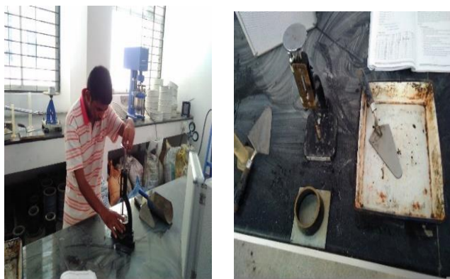
Figure 3.1, 3.2 Vicat apparatus and conducting test on Consistency, Setting time of Cement
