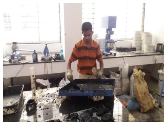
Figure 5.3 Hand mixing of CLSM
