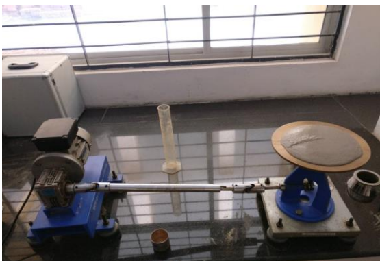
Figure 5.1 Conducting Flow table test
