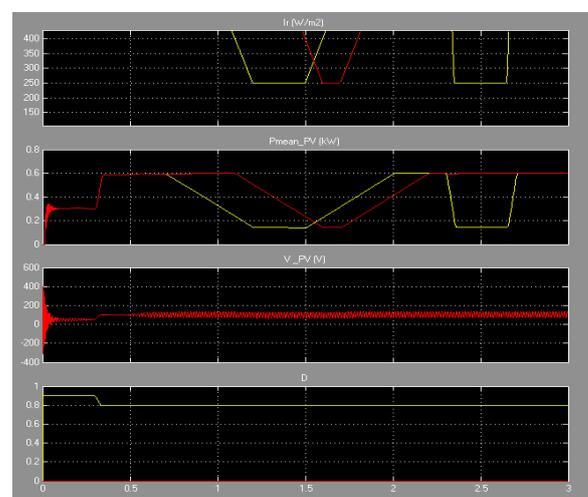
Fig -17: Power output per module for Centralized inverter system
