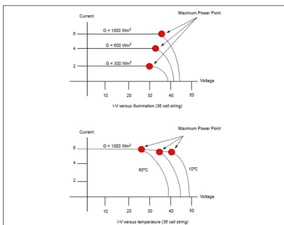
Fig -2 I-V characteristics of PV cell [5]
