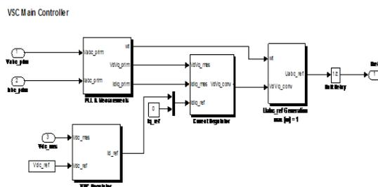
Fig -10: The VSC main controller Simulink model
