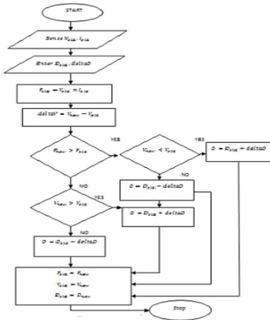
Fig -11: The Perturb and Observe MPPT flow chart
