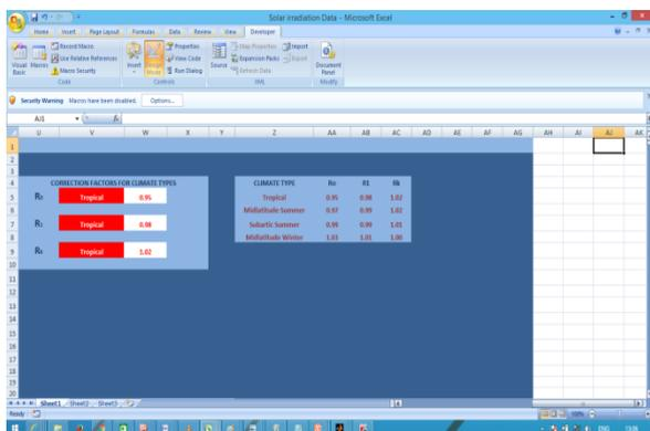
Fig -4: Correction factors for the solar radiation model based on different climatic weather conditions
