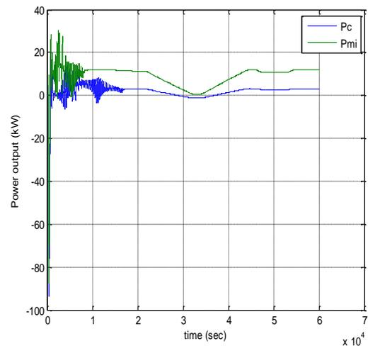
Fig -16: Comparison of power output for centralized and Micro-inverter
