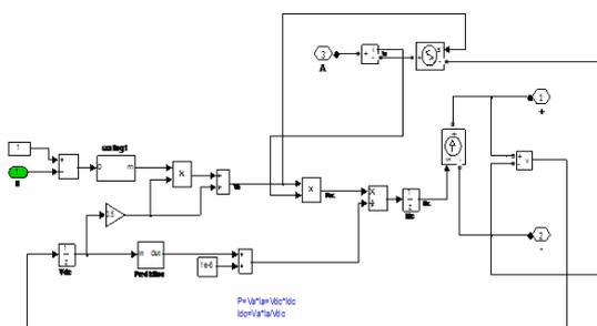
Fig -9: The boost Converter simulink model
