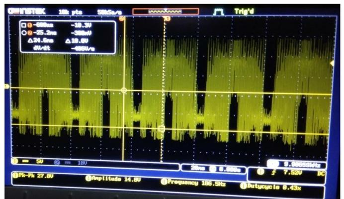
Figure 10 FINAL OUTPUT WAVEFORM
