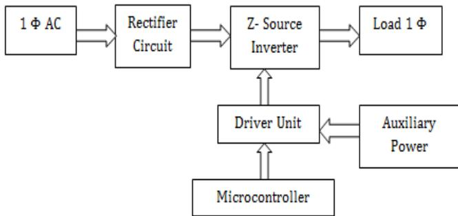
Figure 1: General block diagram of the proposed system
