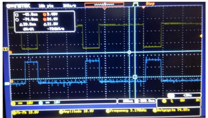
Figure 8 GATE SHOOT THROUGH WAVEFORM
