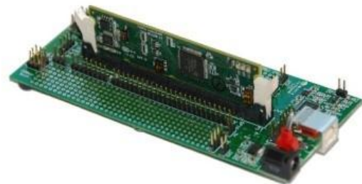
Fig -3. Piccolo F28069 Experimental Kit
