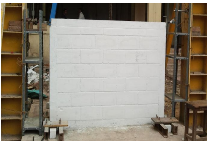
Figure 6: Test set-up for ACB in-fill masonry RC frame
