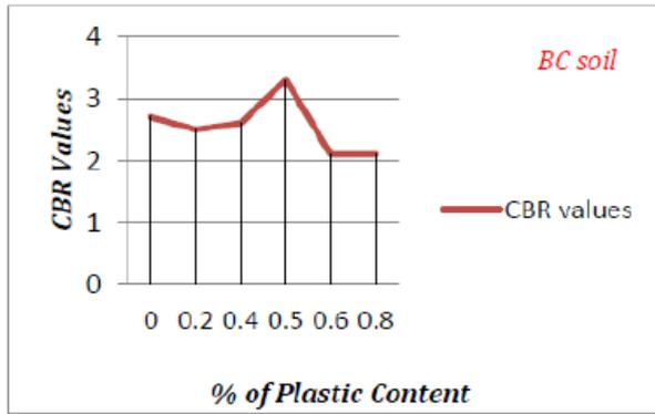
**Figure-2** CBR values of black cotton soil with different % of plastics
