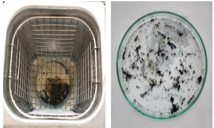
Fig -3: Bathsonicator and dispersion of MWCNT
