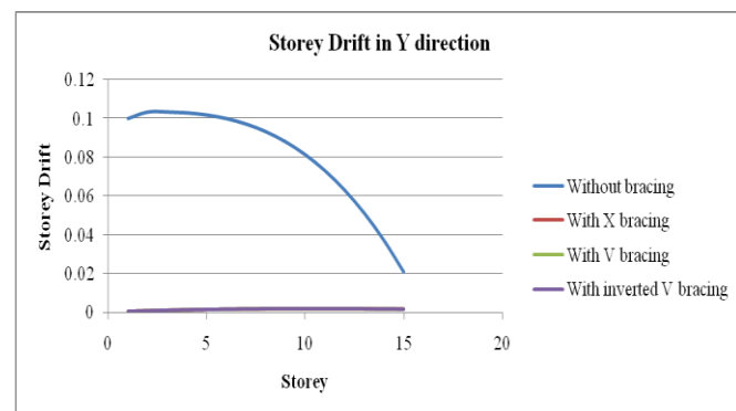
Fig.2.6 Storey Drift in Y direction (G+14)
