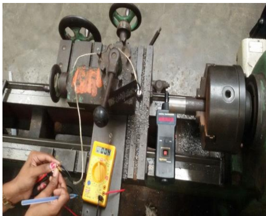
Fig-2 Experimental Set-Up of Tool-Work Thermocouple
