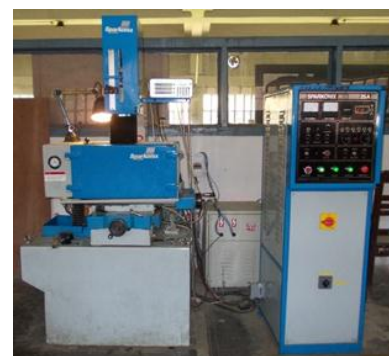
Fig -1: EDM machine set-up
