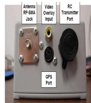
Figure 3 - Antenna Side Ports
