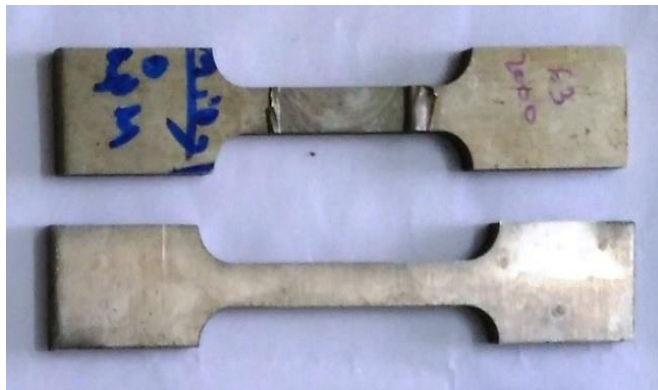
Figure 6 welded and original specimen
