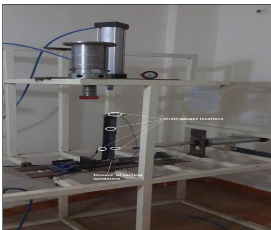
Fig -14: Strain gauge mounted on component with fixture.
