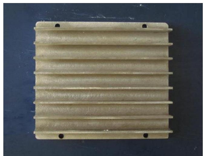
Fig -8: Eight-fin sample with 10.85mm fin spacing
