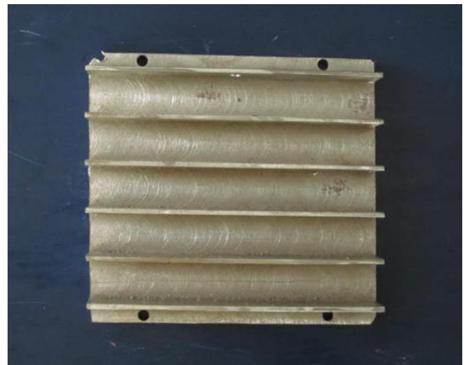
Fig -7: . Six-fin sample with 16mm fin spacing
