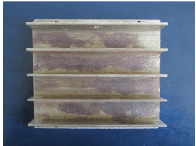
Fig -6: Five-fin sample with 20.5mm fin spacing
