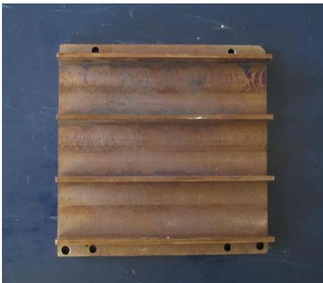
Fig -5: Four-fin sample with 28mm fin spacing
