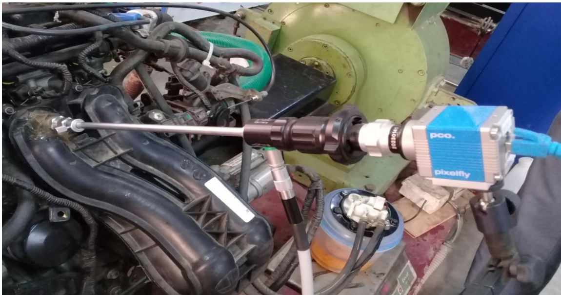
Figure 4 Photographic view of endoscope fitted in test engine
