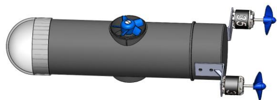
Fig -3: Location of propulsion and dive motors
