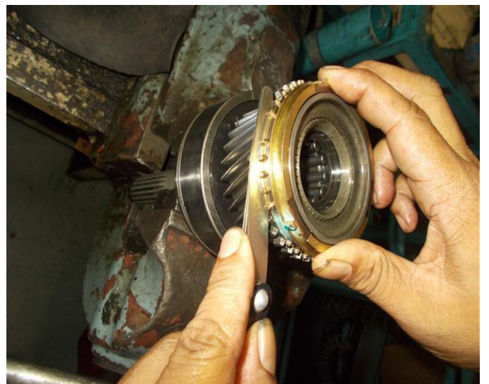
Fig -3: Measurement of clearance
