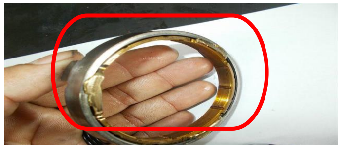
Fig -2: Melted view of synchronizer ring
