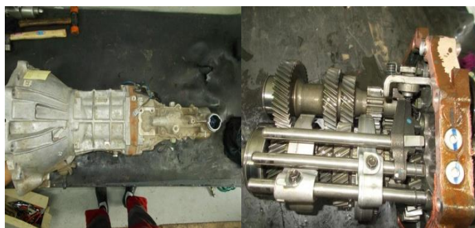
Fig -1: Transmission gear box with gear train
