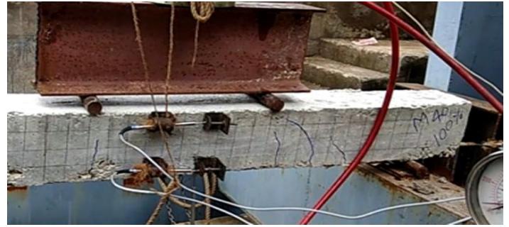
Fig 4.11. Crack profile for RC beam with 100% lapping
