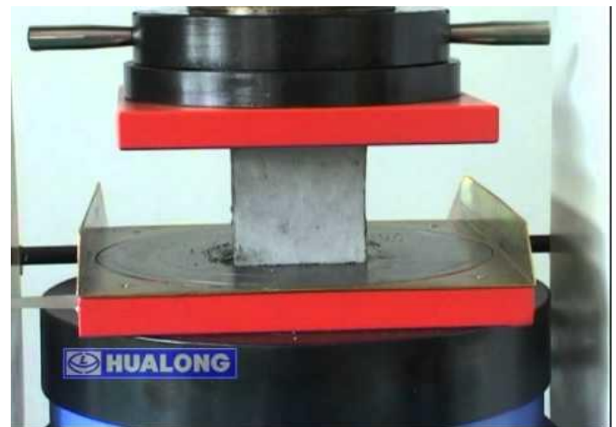
Fig 5. Testing of cube specimen
