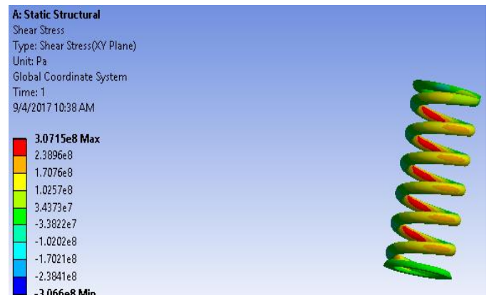
Fig - 5 Shear stress analysis of valve spring
