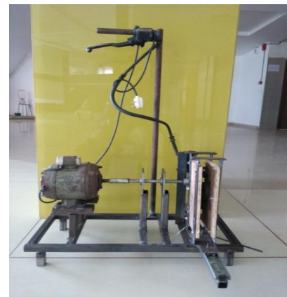
Fig-1 : Fusion braking system
