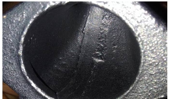
Fig -1: Cold Shut defect in Delivery Casing
