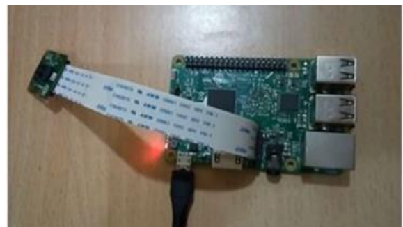
Fig - 6: Manual setup of Vehicle surveillance camera for object detection using Raspicam and Android application
