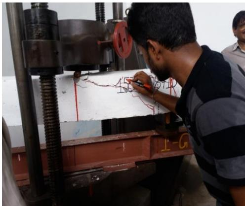
Fig 12: Testing of beam
