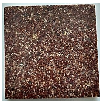
Fig-10: Hardness test specimen of Tamarind shell composite
