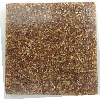
Fig-11: Hardness test specimen of Groundnut shell composite
