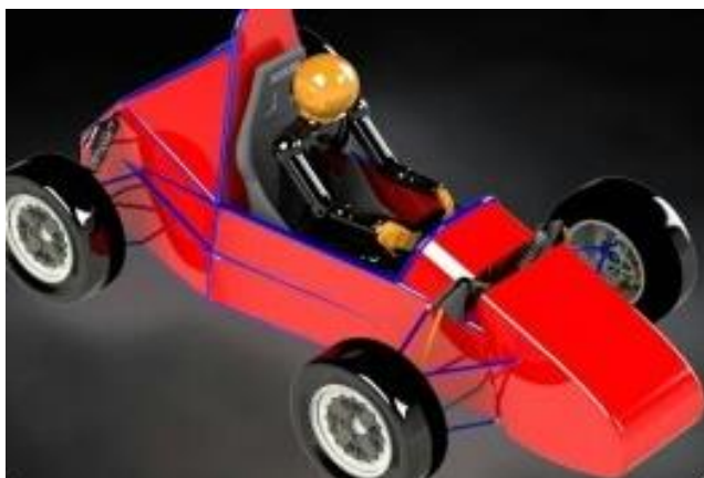
Fig 1: CAD Model of Student formula car
