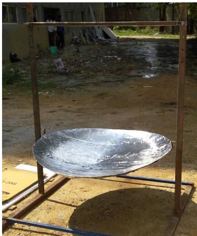
Fig -3: Parabolic reflector with stand.
