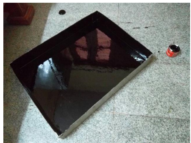
Fig -2: Absorber with aluminium bottom coated with black paint.
