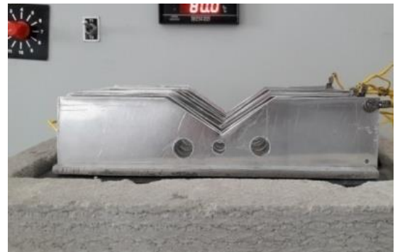
Fig -3: Combination of V-notched (10%) and perforation (10%) fin array
