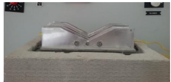
Fig -4: Combination of V-notched (20%) and perforation (10%) fin array
