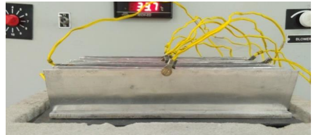
Fig -2: Un-notched (solid) fin array
