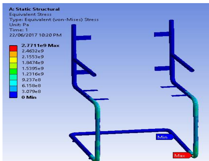
Fig.3: Von- Misses stress for OD=23mm and ID=22mm
