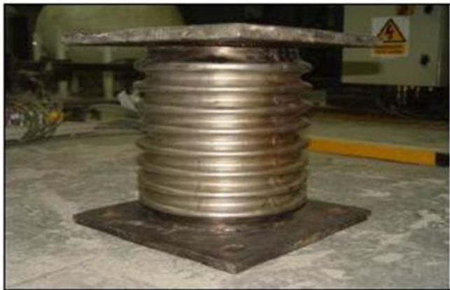
Fig 1.4 Accordion Metallic damper
