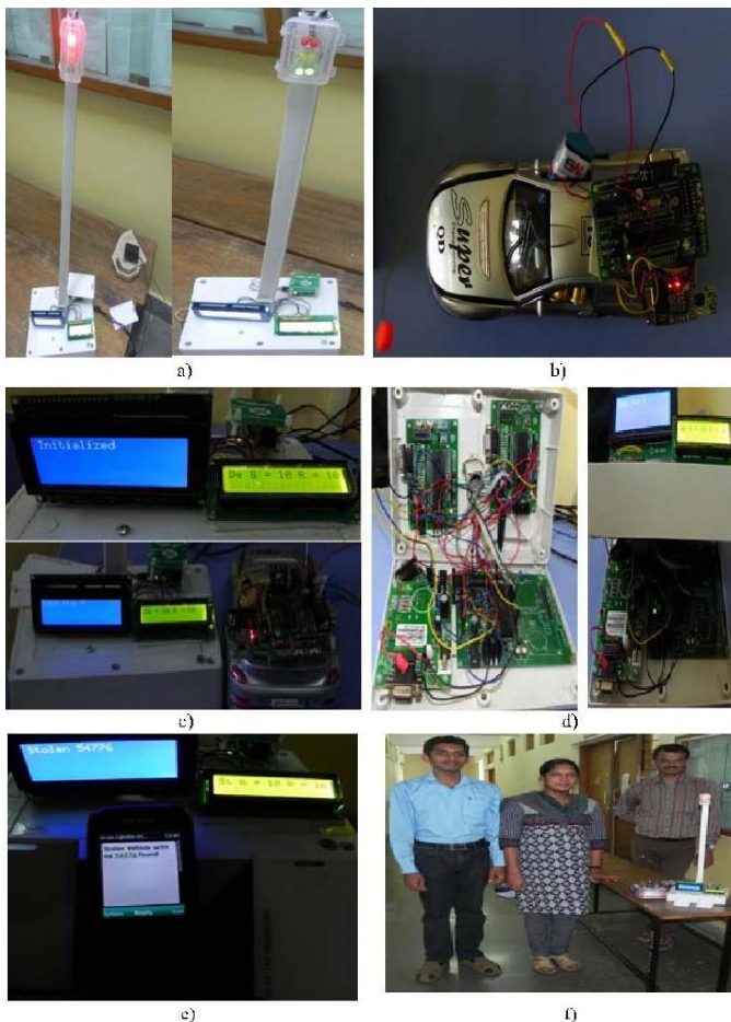
Fig -5: Proposed model images transmitter and receiver. (a) Pole status at different condition. (b) Transmitter (ZigBee). (c) LCD display at receiver.(d) Detailed image of receiver. (e) When stolen vehicle is detected. (f) Working model
