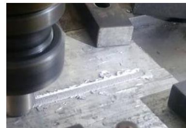
Fig.10 Improved weld after modification
