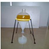
a) Three layered reaction solution in separating funnel.
