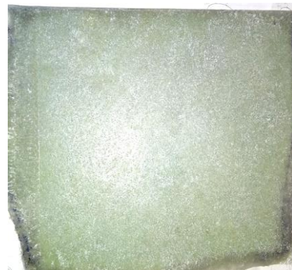
Fig -3: Composite with 10% PTFE filler
