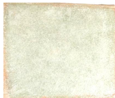
Fig -4: Composite with 20% PTFE filler
