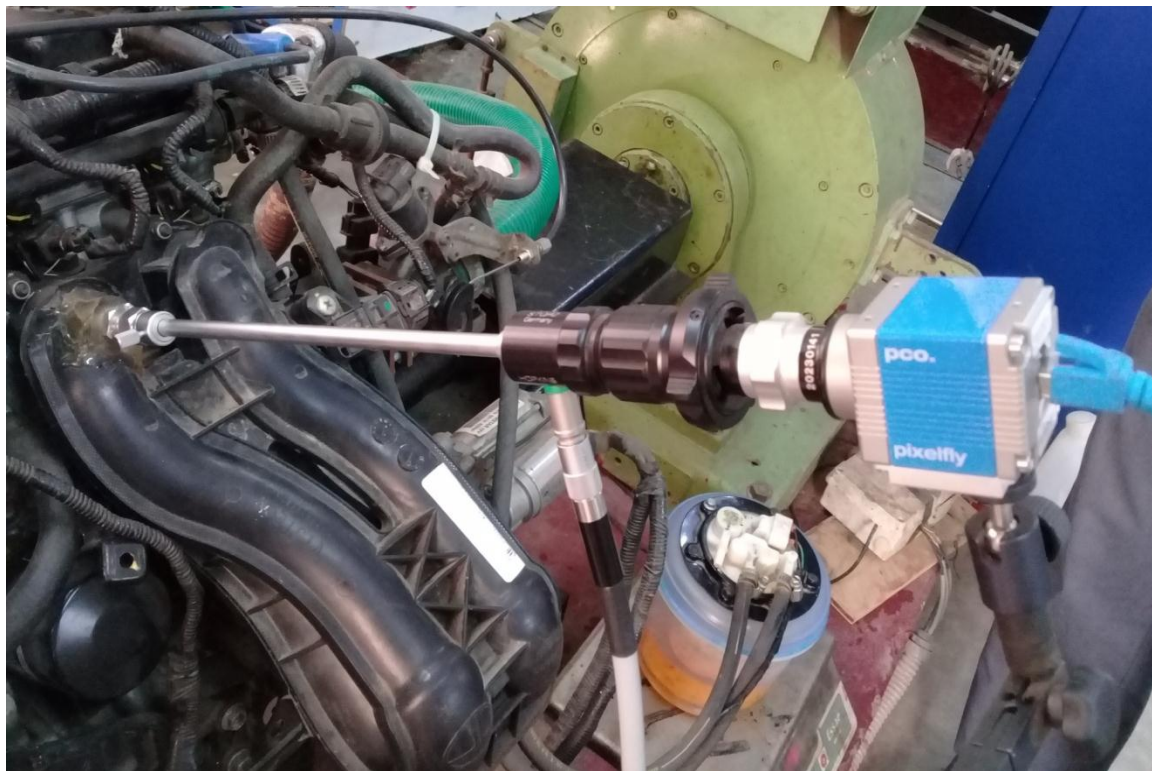
Figure 4 Photographic view of endoscope fitted in test engine
