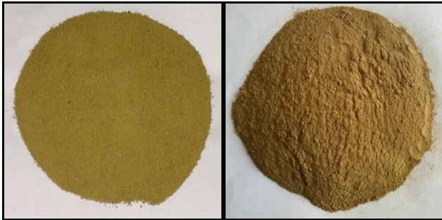
Fig.2: Iron coated bottom ash and iron coated fly ash.
