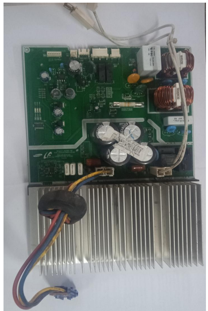
Fig -3: Indoor PCB of Inverter Air Conditioner.
