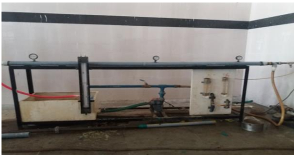
Fig.5: Actual photograph of experimental setup in run mode for 3.81cm pipe diameter
