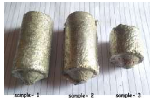
Figure No. 1. - Sample prepared by Stir casting
