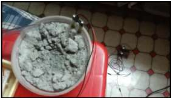
Fig-6: Plant is initially dry (Sample of soil is chosen as a substitute for a full plant as we are concerned with the moisture content of the soil)
