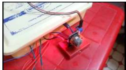
Fig-14: Gas sensor to detect gas leak
