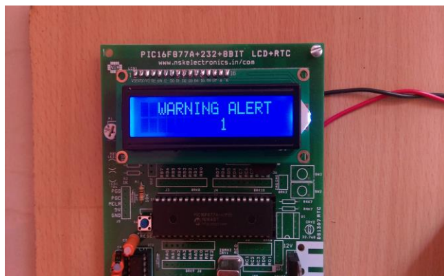
Fig - 8: LCD Display during Emergency Condition.
