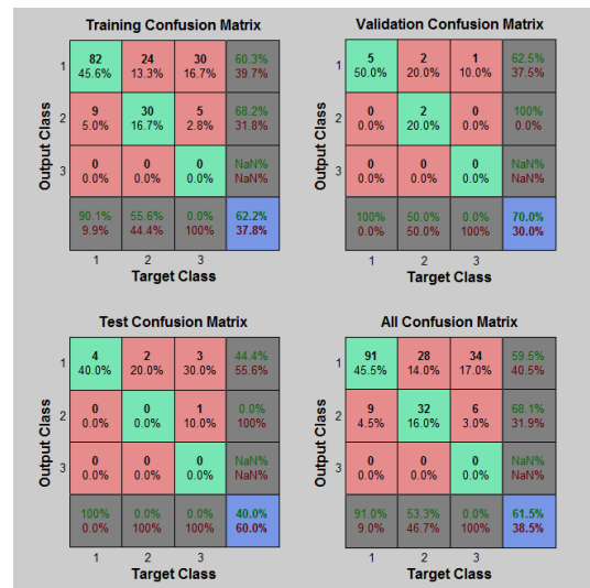
Fig-15: Confusion matrix after successful training of ANN2 for transmission line fault zone identification.
