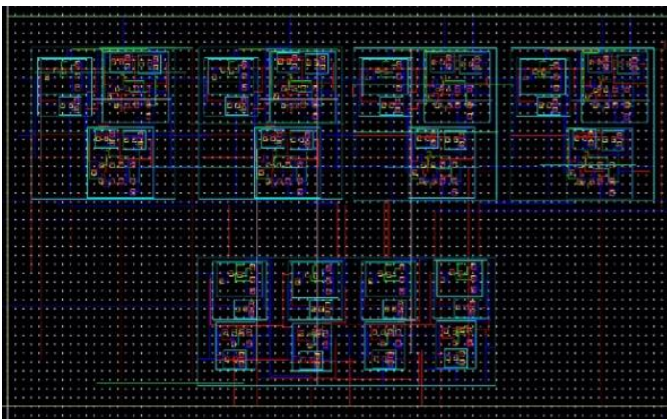
Fig-23: Layout of an adiabatic 2PASCAL 4-bit carry-lookahead adder.
