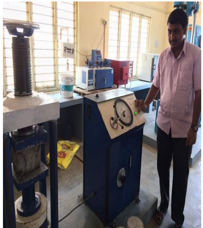
Fig -1: Compression strength test of cubes
