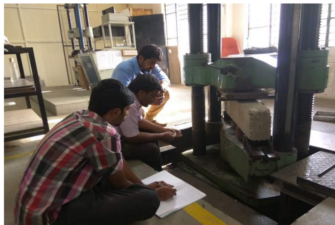
Fig -5: Flexure test of beams
