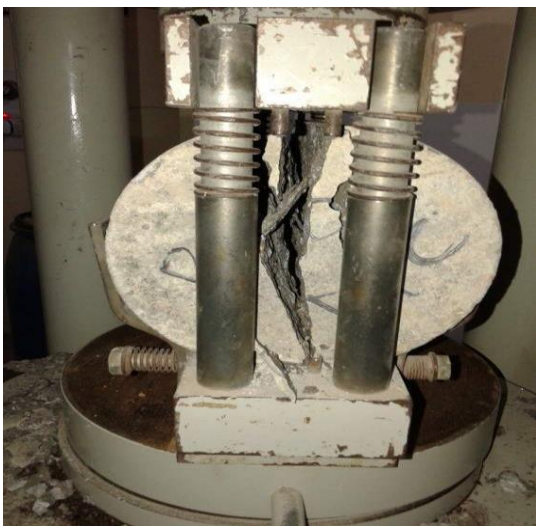
Fig -2: Split Tensile test of cylinders
