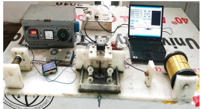
Fig-2: In house fabricated TW-ECDCM setup
