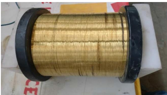
Fig-4: Zinc coated brass wire
