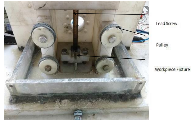
Fig-5: Job fixture to hold the workpiece
