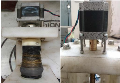
Fig-3: Wire winding & workpiece feeding stepper motors
