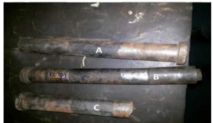
fig. failure of knuckle pin
