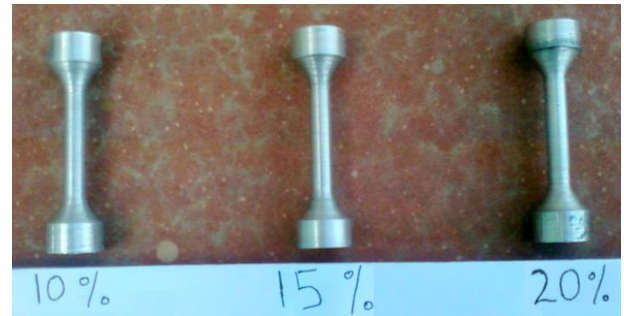
Fig(2): Tensile Strength Specimens of different composition
