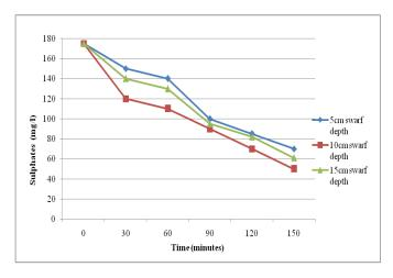
Fig 3.5: Variations of Sulphates in 5cm, 10cm and 15cm swarf depth.
