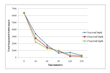
Fig 3.2: Variations of Total Suspended Solids in 5cm, 10cm and 15cm swarf depth.
