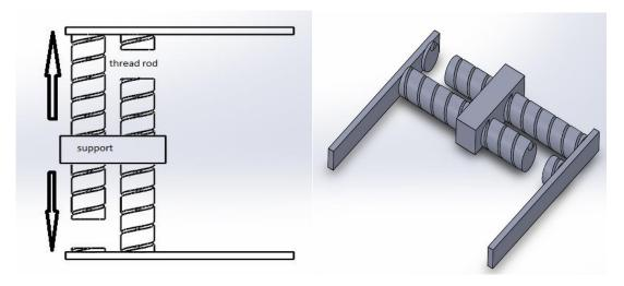
Fig 4.1 and 4.2 top and isometric view of horizontal adjustment
